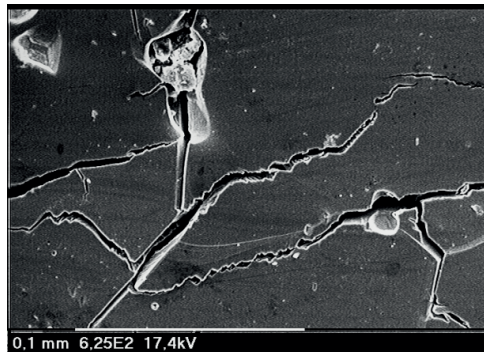
Fig. 11. Microstructural observations of type B of NiAlTiB alloy by scanning electron microscope, temperature of 673 K, \varepsilon = 0.07
